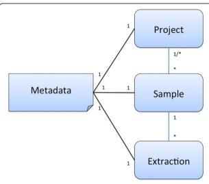
Figure 4 A three-tiered hierarchy allows modeling of real-life experiments, combining multiple "samples" into a "project" (or study) and allowing for different "extractions" from the sample.
